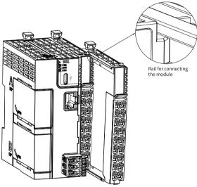
Install an DIN rail end plate to both sides of the master or module. To mount the end plate, hook the bottom of it to the bottom of the DIN rail, rotate the end plate to hook the top of it to the top of the DIN rail, and then tighten the screw to lock the end plate in place, as shown below.
