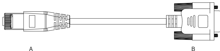
Figure 3-45 Outline drawing of the PC communication cable
